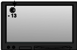
Fig. 28: Display with pointer symbol and number of degrees
