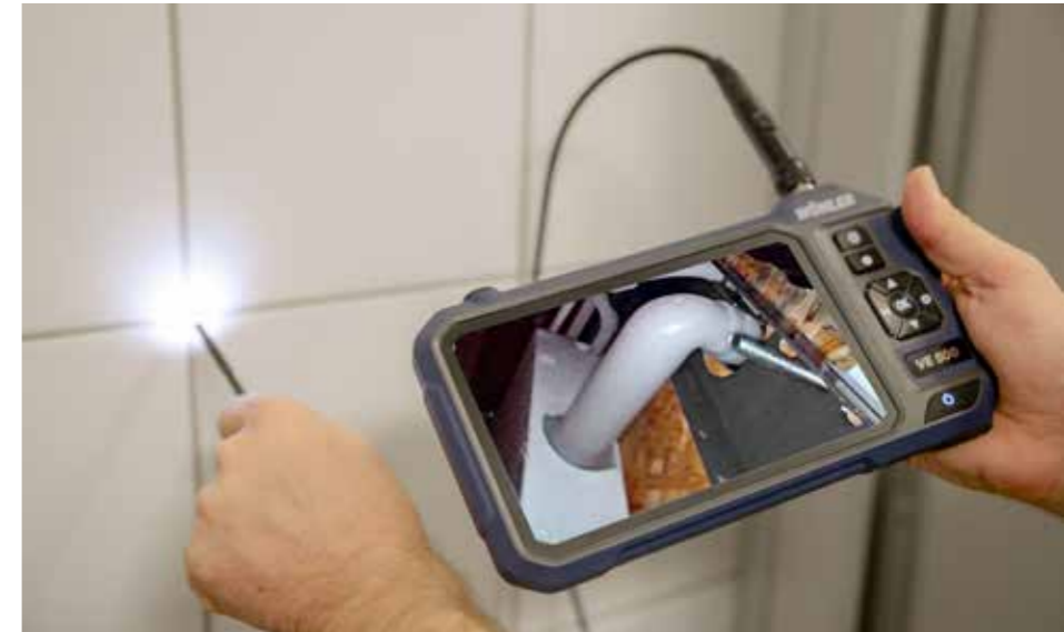
A Ø 6 mm opening in a tile cross is sufficient to inspect the installation behind the wall.
