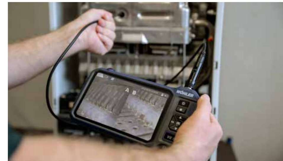
The split-screen mode allows you to display both camera images of the combination probe simultaneously to capture everything at a glance.
