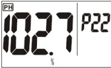
Fig. 51: Slope value within permissible range
