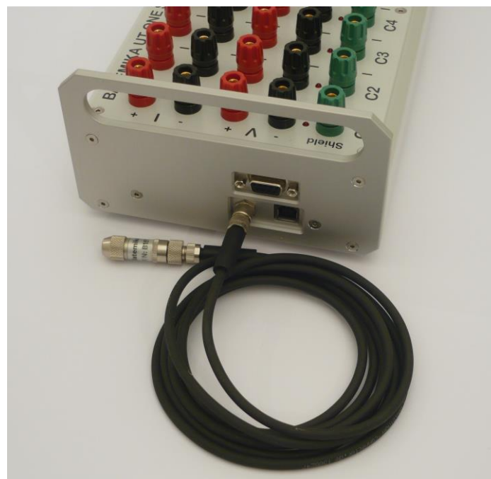
Connection of ambient probe using 2 m extension cable
