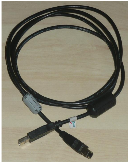
Figure 22: USB cable with ferrite cores
