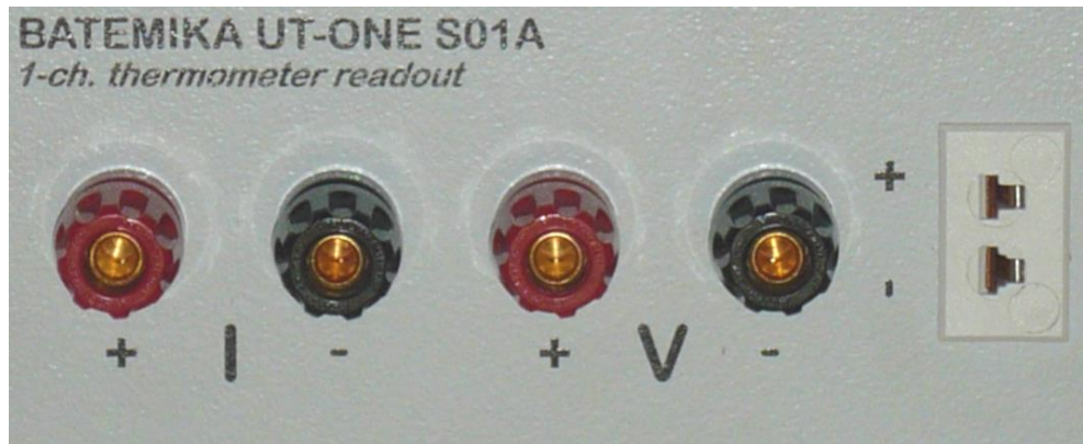
Figure 2: Connectors for the connection of thermometer probe on main channel
