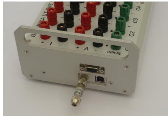
Ambient probe connector with plastic protective plug, direct connection of ambient probe
