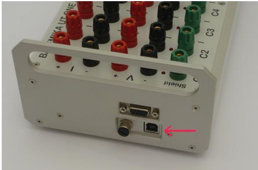
Figure 16: USB connector on the side panel of UT-ONE
