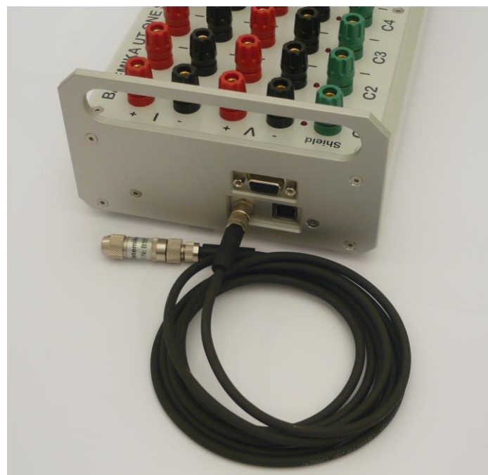
Connection of ambient probe using 2 m extension cable
