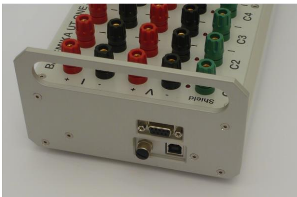
Ambient probe connector with plastic protective plug, direct connection of ambient probe
