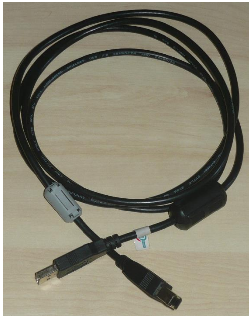
Figure 21: USB cable with ferrite cores
