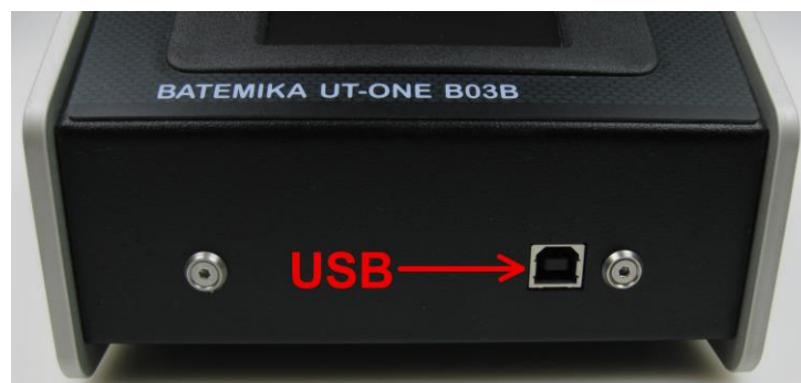
Figure 51: USB connector on the front side of UT-ONE B03B
