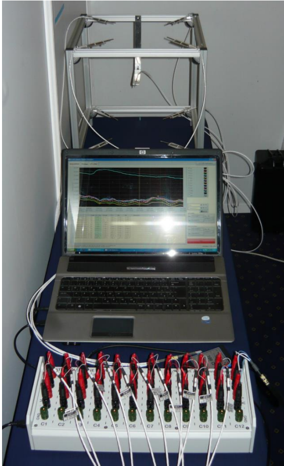
Demonstration of validation of climatic chamber with UT-ONE S12A, 12 Pt-100 probes and computer with acquisition software
