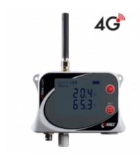
GSM Datalogger is designed to record temperature from two external Pt1000 probes. In case of exceeded set limits, SMS and JSON messages can be sent via 4G data connection. Measured values can be sent to the internet storage  $\underline{\mathsf{COMET\ Cloud}}$ , which is a complete monitoring, alarm and analysis system.
