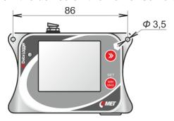
You can fix the device on the wall with the aid of a lockable holder LP100 (optional accessory)
