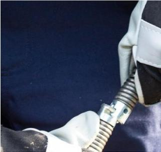
Fig. 8: Fixing the auger with the snap-lock
