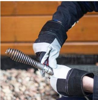
Fig. 9: Releasing the snap lock to separate the drill head from the cable.
