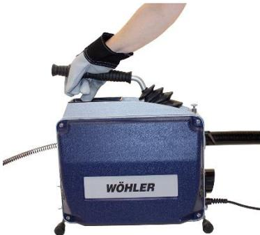
Fig. 5: Control handle down: cable rotates
