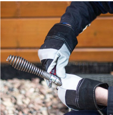
Fig. 7: Releasing the snap-lock to separate the drill head from the cable.
