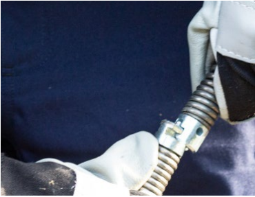
Fig. 6: Fixing the drill head with the snap-lock
