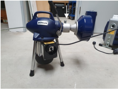
Fig. 11: Adapter attached to the RM 200, locking bolt marked by an arrow
