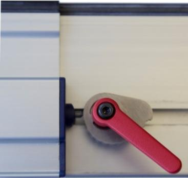
Fig. 21: Tensioning the frame
