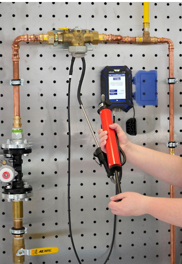
Fig. 44: Manual volume measurement with a Wöhler M 603 and a soot test pump
