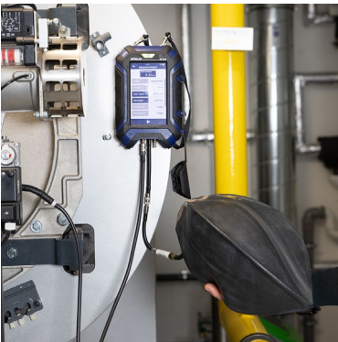
Fig. 5: Connection of the Wöhler M 603 for automatic usability measurement with filled gas bellows
