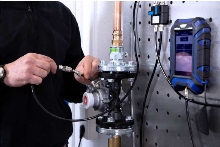
Fig. 47: Flexible adapter screwed onto the gas regulator
