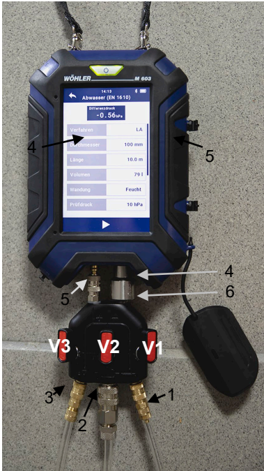
Fig. 72: Valve block with connections to the Wöhler M 603, to the air pump, and to the inflatable sealing bladder
