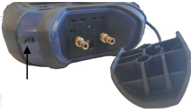
Fig. 4: Protective cover for pressure connections; the protective plugs are marked with an arrow
