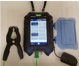
Fig. 10: Connection of a temperature clamp probe
