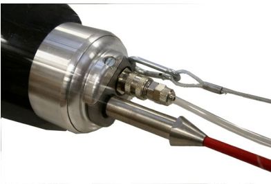
Fig. 74: Pulling off the push rod
