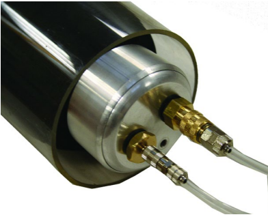
Fig. 77: Test bladder with measuring hose and hose to the air pump
