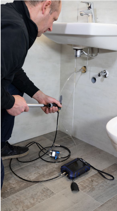
Fig. 58: Connection example using the Wöhler leak tightness testing set for gas pipes for the stress test
