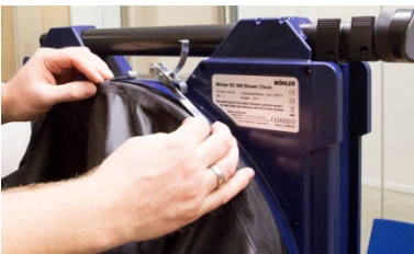
Fig. 12: Pull fan strap around the edge of the blower fan
