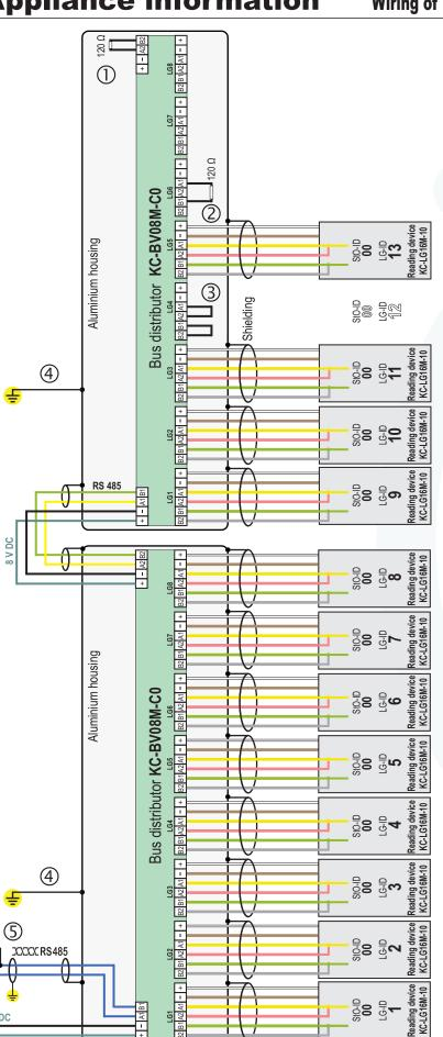
Please insert the enclosed termination resistor 120  $\Omega$  at the end of the bus cable:
