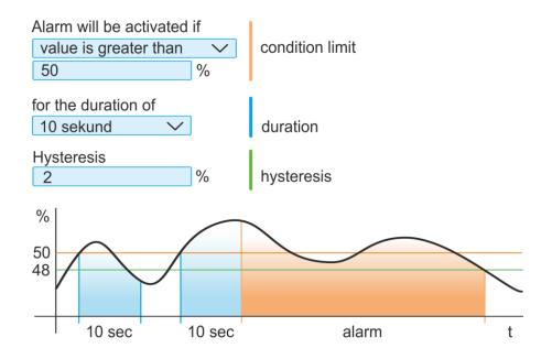
Thus, the setting for generating an alarm is completed. It remains to decide, whether the alarm should be indicated optically by means of a LED diode on the device (*Optical signalling - LED*) or acoustically (*Activate internal acoustic signalling*)
