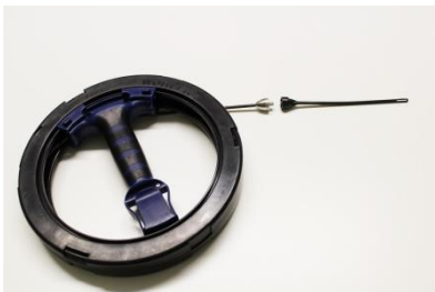
Fig. 14: Screwing the Push rod onto the viper
