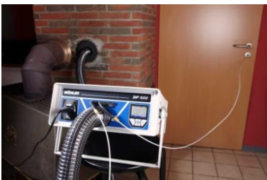
Fig. 57: Wöhler DP 600 with capillary hoses during the 4 PA test.
