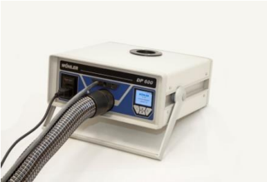
Fig. 30: Hoses and cable connected to the measuring instrument for the leakage test class N: Mains cable, pressure hose and plastic hose
