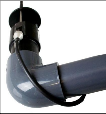
Fig. 31: Probe connected to the extension pipe.
