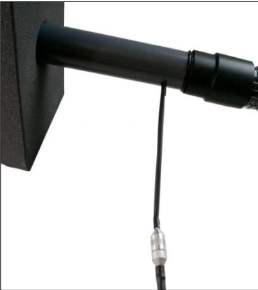
Fig. 31: Probe connected to the extension pipe.
