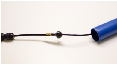
Fig. 22: Connection of the two sealing bladders
