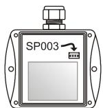
when new setting is saved and finished, disconnect the cable from the device, connect wires into its terminals and place the lid back to the device
