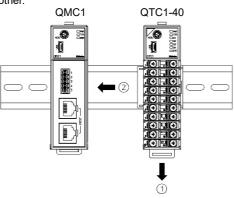
3 Raise the lock lever of the QTC1-40. Make sure it is fixed to the DIN rail.
