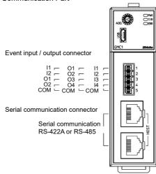
(1) Pin arrangement of event input / output connector Using the event input/output connector [0225-0805 (DINKLE)] (sold separately).
