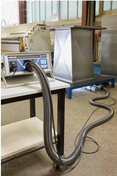
Fig. 12: Example: Measurement according to DIN EN 15727
