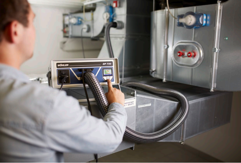
Fig. 11: Example: positive pressure measurement without adapter
