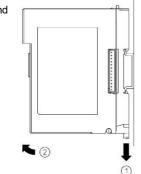
Mounting multiple modules to the DIN rail
