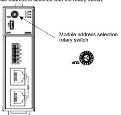
Use a small flat blade screwdriver to select the module address The module address of QMC1-C□ differs depending on the model
