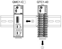
3 Raise the lock lever of the QTC1-40. Make sure it is fixed to the DIN rail.
