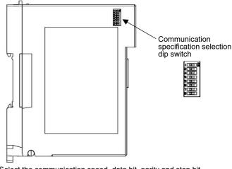
Select the communication speed, data bit, parity and stop bit. All are off when shipped from the factory.
