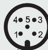
Circular connector M12 x 1, 5-pin
