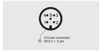
Connect the cable shield to the force transducer housing. In the case of accessory cables, the cable shield must be connected with the knurled nut and thus connected to the housing of the force transducer. When extending, only shielded and low capacitance cables should be used. The permitted maximum and minimum lengths of the cable are specified in ISO 11898-2. A high-quality connection of the shielding must also be ensured.
