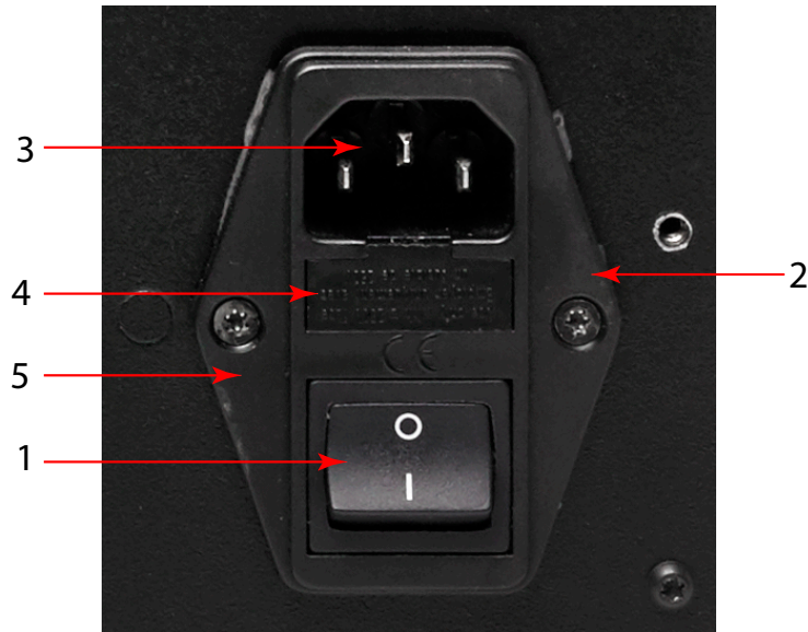
Figure 27 Power Supply Fuse Replacement
