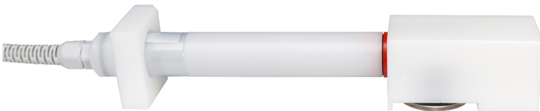
Figure 8: Calibration device with installed HM4 probe.
