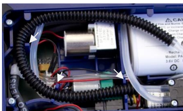
Fig. 73: Corrugated tube, correctly positioned, guiding hooks marked by an arrow.
