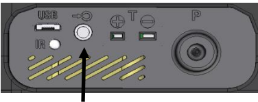
Fig. 39: Connectors for the wood moisture probe at the bottom of the analyzer
