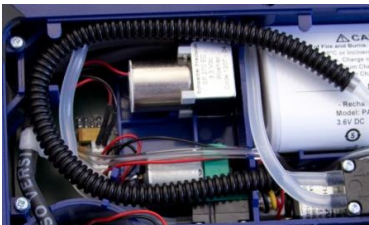
Fig. 75: Corrugated tube, correctly positioned
