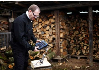
Fig. 40: Wood moisture measurement with Probe Wöhler HBF 420.
