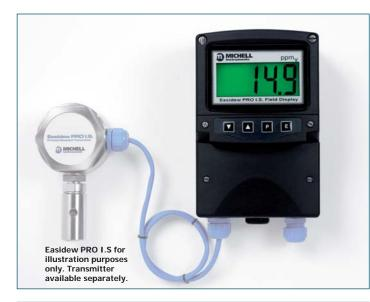
The Intrinsically Safe Field Display is a 4-digit loop-powered local monitor for the Easidew PRO I.S. and Easidew I.S. transmitters. It is certified with ATEX, IECEx, and FM and housed in an IP66 enclosure with a terminal compartment for wiring. The measurement unit can be labelled as  $ppm_{v'}$   $ppm_{w'}$  °C dp or °F dp.
