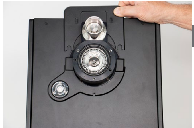
Figure 8.1.3.4-A Trim Plate Removal
