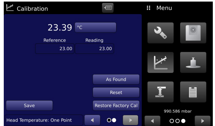
Figure 8.2.6.1-D Saving One Point Calibration
