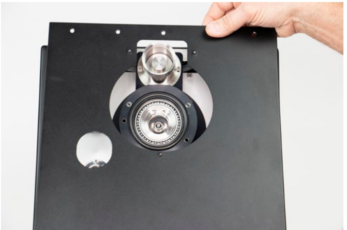
Figure 8.1.3.4-B Top Cover Removal
