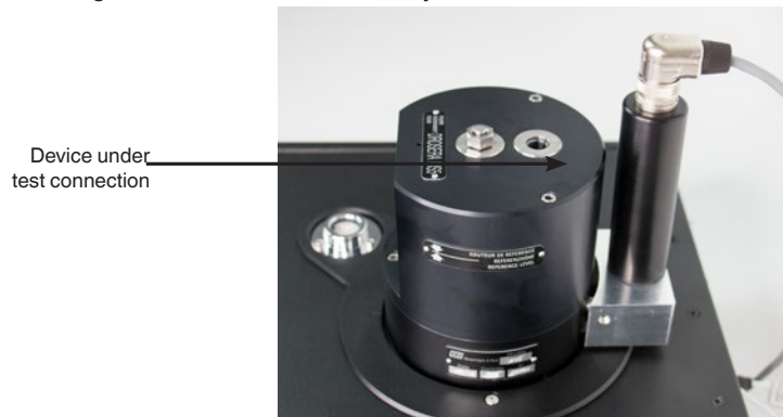
Figure 5.6.3 Gauge Pressure Connections
