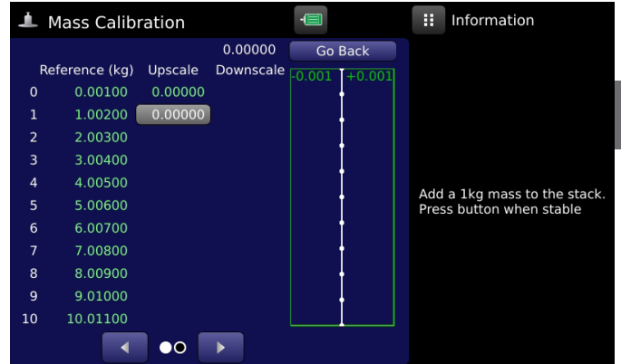
Figure 8.2.7-F Upscale Mass Adjustment
