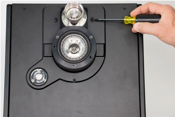
Figure 8.1.3.4-A Trim Plate Removal
