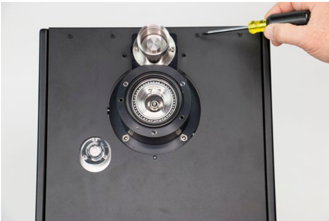
Figure 8.1.3.4-B Top Cover Removal
