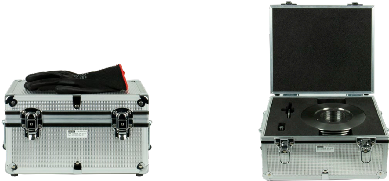
Figure 11.7 External Mass Set in Carrying Case
