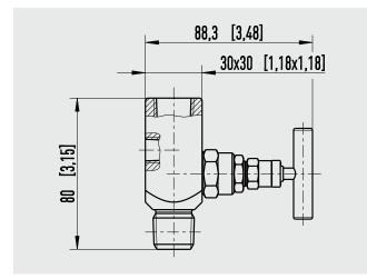
Plug screw for vent connection is included in delivery, though not pre-fitted.
