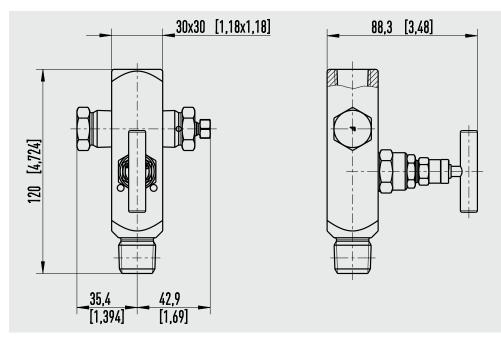
Plug screw and vent screw is included in delivery, though not pre-fitted.
