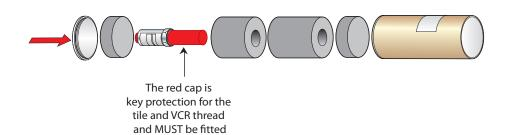
If the sensor is returned without the red cap fitted and/or damage is found on the threads, the contract will be void.
