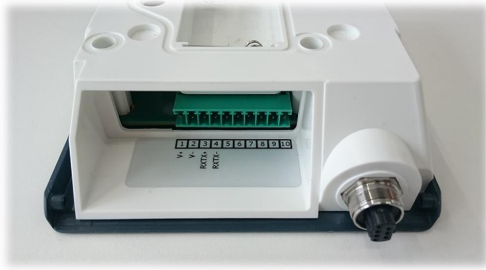
Figure 5: Electrical connections of the data logger
