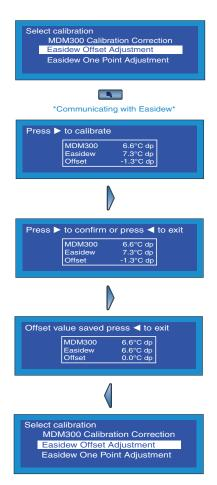
Figure 35 Easidew Offset Adjustment
