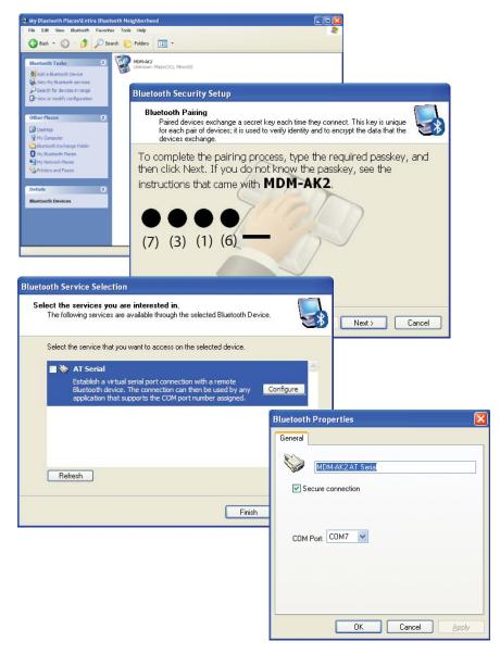
Figure 20 Typical Bluetooth Pairing Sequence
