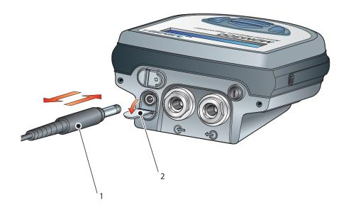
Figure 14 Battery Charger Connection
