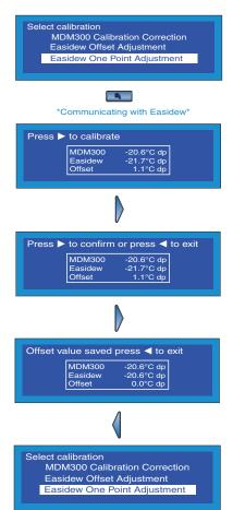
Figure 36 Easidew Single Point Adjustment
