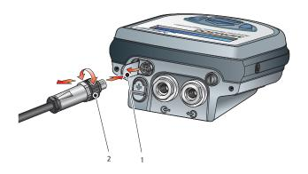
Figure 9 External Transmitter Connection
