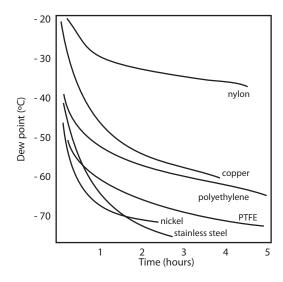
All materials are permeable to water vapor, as the water molecule is extremely small compared to the structure of solids, even when compared to the crystalline structure of metals. The graph to the right shows the dew point inside tubing of different materials when purged with very dry gas, where the exterior of the tubing is in the ambient environment.
