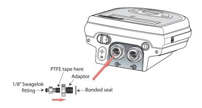
Figure 7 Bonded Seal Fitting
