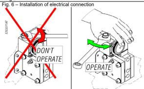
With the instrument into the final position provided that the electric line is not energize, remove the cover and make the electrical connection to the terminal block (see Fig. 2)
