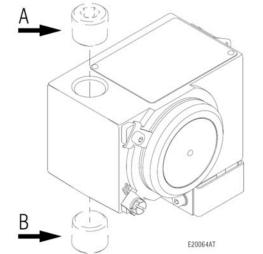
CAUTION: fittings used for the electrical connection of the flameproof instruments shall be certified according the IEC or EN standards and shall guarantee instrument degree of protection (IP66).
