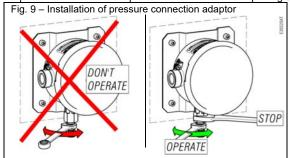
**Carry out** the connection to the process using a flexible tube in such a way that variations in the temperature of the tube itself do not force the instrument attachment.
