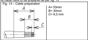
The single stripped conductor has to be crimped with each contact pin. For the electrical connections and for the assembly follow Fig 14
