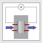
The MSRS responds quickly to oxygen and has a T90 of under 11 seconds. Another benefit of having a sealed reference is that measurements can be made without a reference gas and independent of the quality of the surrounding air. The analyzer is virtually drift-free, extending calibration interval time.
