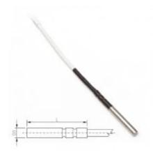
Multi-purpose watertight IP67 probe -190 to  $+150^{\circ}$ C. Accuracy class B. Stainless steel 17240 with teflon cable of specified length, with CINH connector. Diameter 5  $\pm$  0.1 mm, length 50mm.
