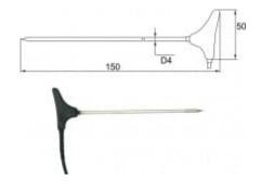
Temperature probe with Pt1000 sensor.
