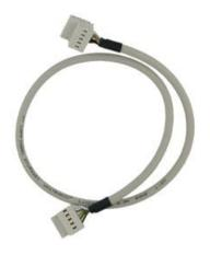
Connection cable for MP016 terminal with display and MP018 output relays module - cable length approximately 60cm. Longer cable lengths available - maximum 2m for relay module, maximum 50m for the terminal with display.
