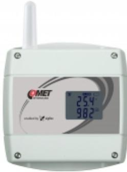
The device measures the temperature and concentration of CO<sub>2</sub> from an internal sensors.
