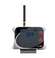
GSM datalogger is designed to record from four binary inputs or from two pulse and two binary inputs. In case of exceeded set limits, SMS and JSON messages can be sent via GPRS data connection. Measured values can be sent to the internet storage <a href="COMET Cloud">COMET Cloud</a>, which is a complete monitoring, alarm and analysis system.
