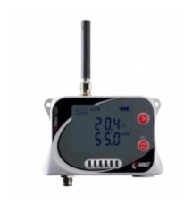
GSM datalogger is designed to record temperature and humidity from built-in sensors and temperature from external probe. In case of exceeded set limits, SMS and JSON messages can be sent via GPRS data connection. Measured values can be sent to the internet storage <a href="COMETCloud">COMETCLOUD</a>, which is a complete monitoring, alarm and analysis system.
