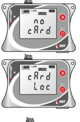
Displayed when no SIM card is inserted
