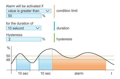
Thus, the setting for generating an alarm is completed. It remains to decide, whether the alarm should be indicated optically by means of a LED diode on the device (*Optical signalling - LED*) or acoustically (*Activate internal acoustic signalling*)
