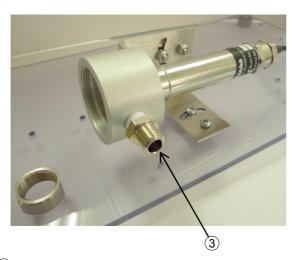
3 Connect a tube, connector or pump to the air purge collar.
