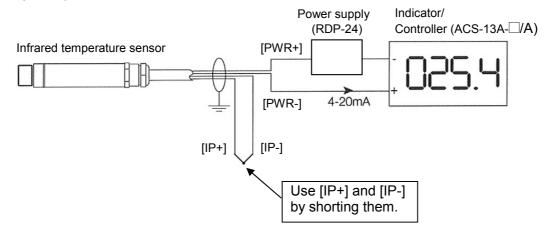
Emissivity can be set on the ACS-13A-\(\triangle A\).
