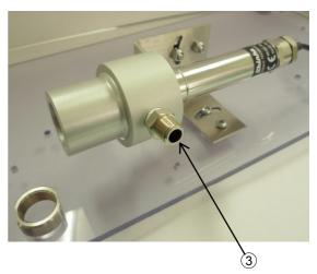
③ Connect a tube, connector or pump to the air purge collar.
