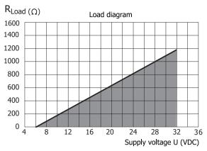
Maximum load depending on power supply Formula for the max. permissible output load for APAQ C130:
