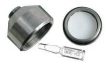
Accessory is designed to verify the measuring accuracy (calibration) and new adjustment of instruments sensing the air relative humidity. Relative humidity is generated in air-tight vessel fixed to relative humidity probe. The value of relative humidity is depends on chemical solution applied inside of the vessel.
