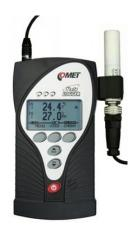
Battery powered datalogger for external CO2 probe up to 10 000ppm or 50 000ppm and inputs for connecting up to three temperature and/or humidity probes.
