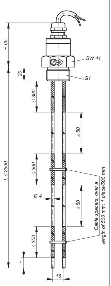
\* 8 % of the electrode rod length, however min. 10 mm
