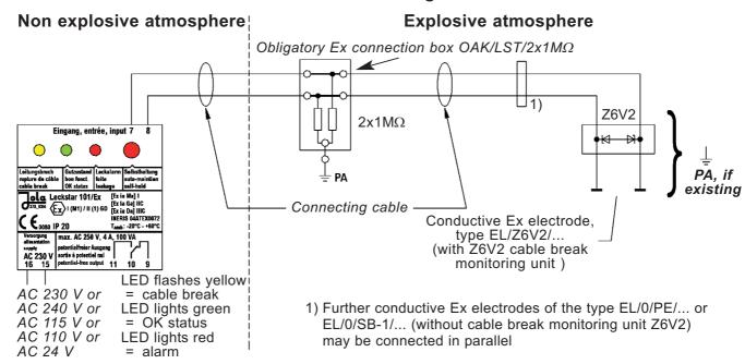
Position of contact when Leckstar 101/Ex without voltage
