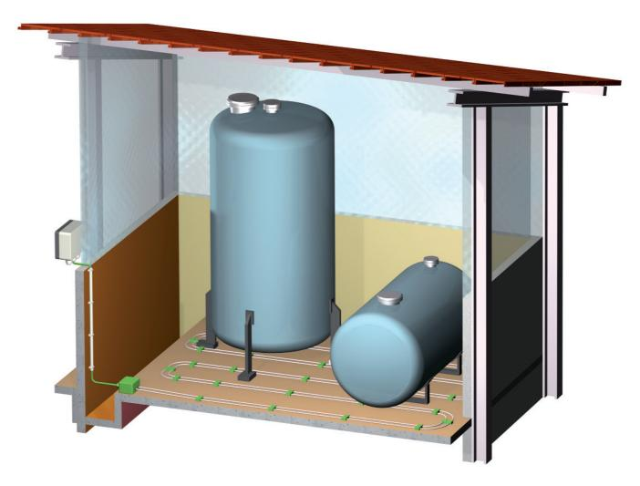
Use of an Ex cable electrode for leakage detection of a conductive liquid in a storeroom
